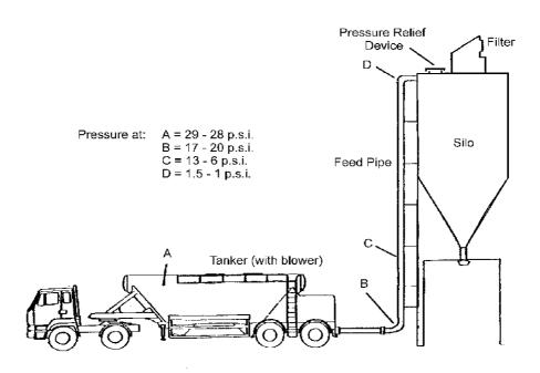
Figure 3. Schematic representation of the delivery system, with typical pressures measured in the delivery pipe.
