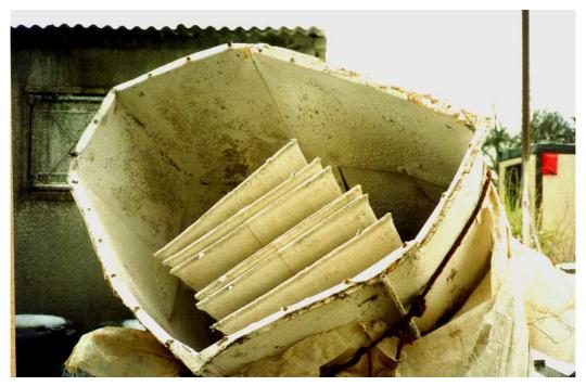
**Figure E1.** Filter housing which has been ejected from the top of a silo. The bolts holding the housing in place have been torn through the metal flange.
