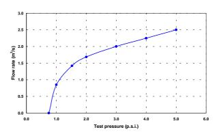
**Figure B1**. Plot of PRV operating characteristics (based on information from manufacturer).
