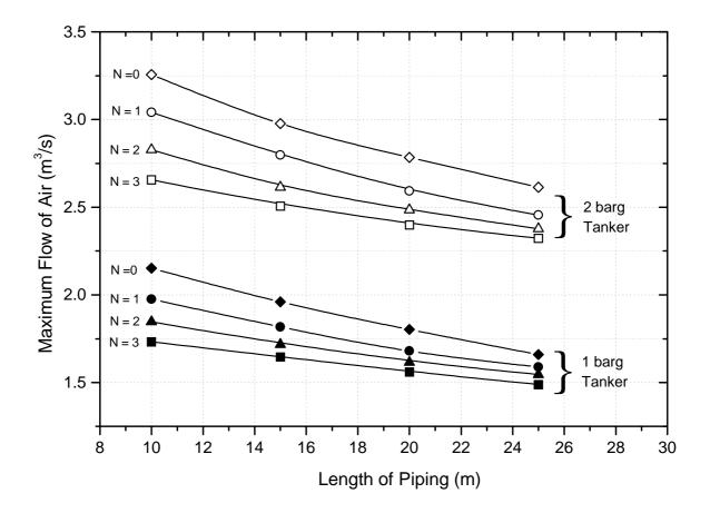
Figure A1. Plot of maximum discharge rates against length of piping (diam. = 4" (100 mm)) for tanker pressures of 1 and 2 barg, and for pipes containing up to three  $90^{\circ}$  bends (N = 0, 1, 2, or 3).
