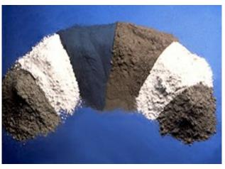
Supplementary cementing materials. L-R: Fly ash (TypeCI), metakaolin (calcined clay), silica fume, fly ash (Type F), Slag, and calcined shale.
