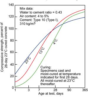
Rate of setting and strength gain can be increased by increasing the cement content of a concrete mix or by using a Type HE cement. The quantity or fly ash or slag in concrete may be reduced for a similar effect. However, this may not be possible if a minimum quantity of SCM is required for durability such as for sulphate resistance or mitigation of ASR. The selected solution should be economical and not compromise on the required concrete performance.
