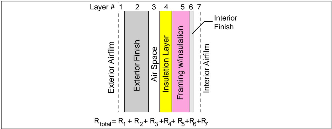
Figure 7: Example calculation of multi-layer assembly thermal resistance.
