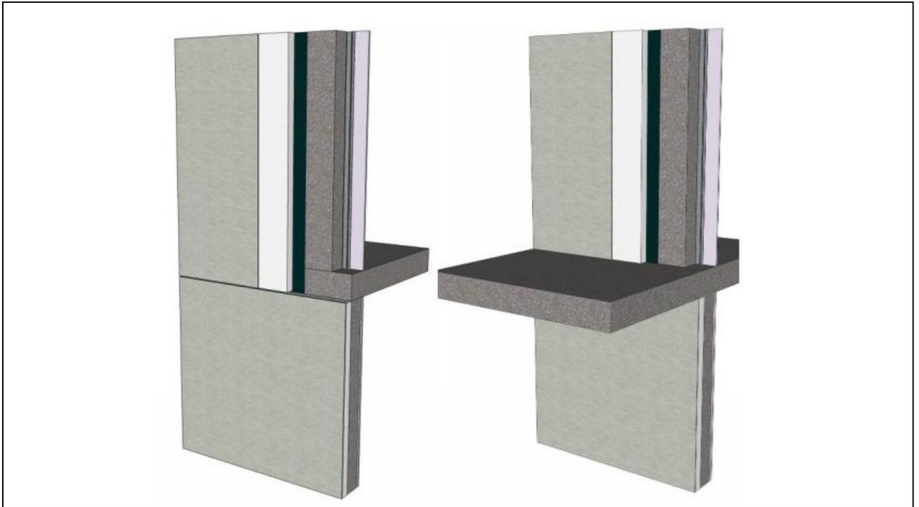
*Figure 17: Exterior insulated CIP wall system at floor slab intersection (RDH 2013).*
