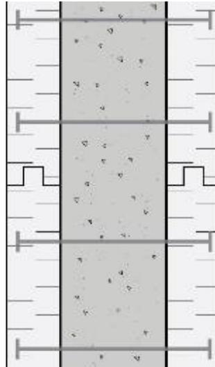
Figure 22: Generic cross-section through an ICF wall.
