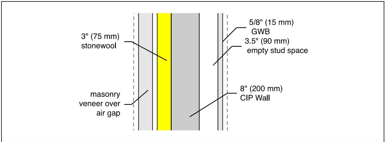
Figure 14: Example exterior insulated CIP wall with masonry veneer.
