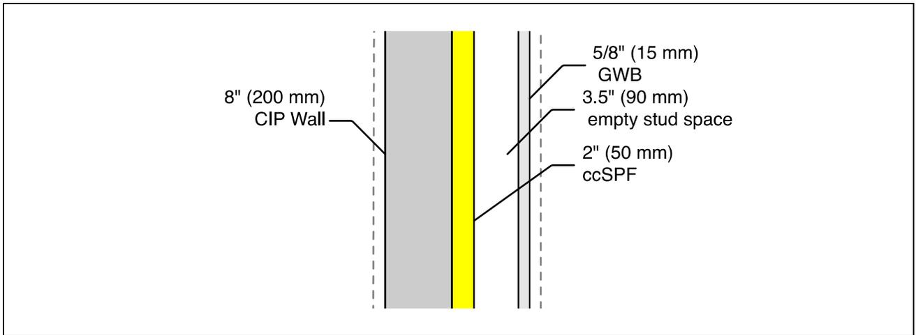
Figure 13: Example interior insulated CIP assembly.
