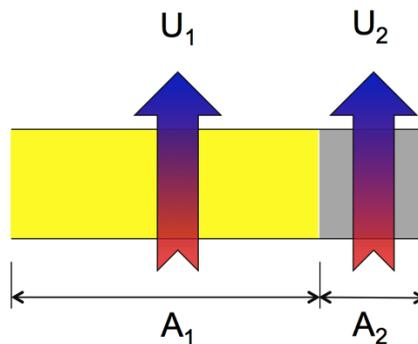
Figure 8: Parallel path heat flow.
