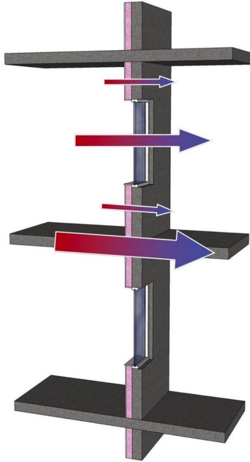
*Figure 4: Heat flow paths through center of wall, floor slab, and windows (arrow size is relative to magnitude of heat flow).*
