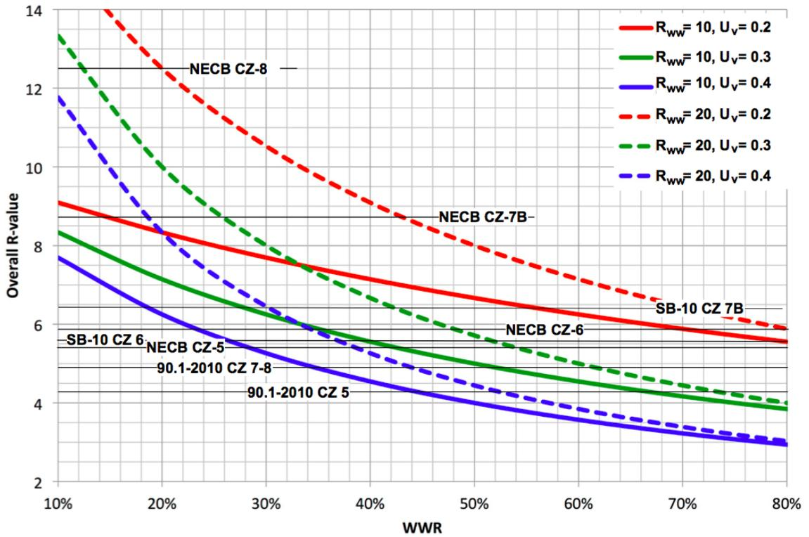
Figure 10: Overall R-value of mass walls and metal windows and the WWR (Note: CZ= climate zone,  $R_{ww}$  is whole-wall R-value, and  $U_v$  is window U-value).
