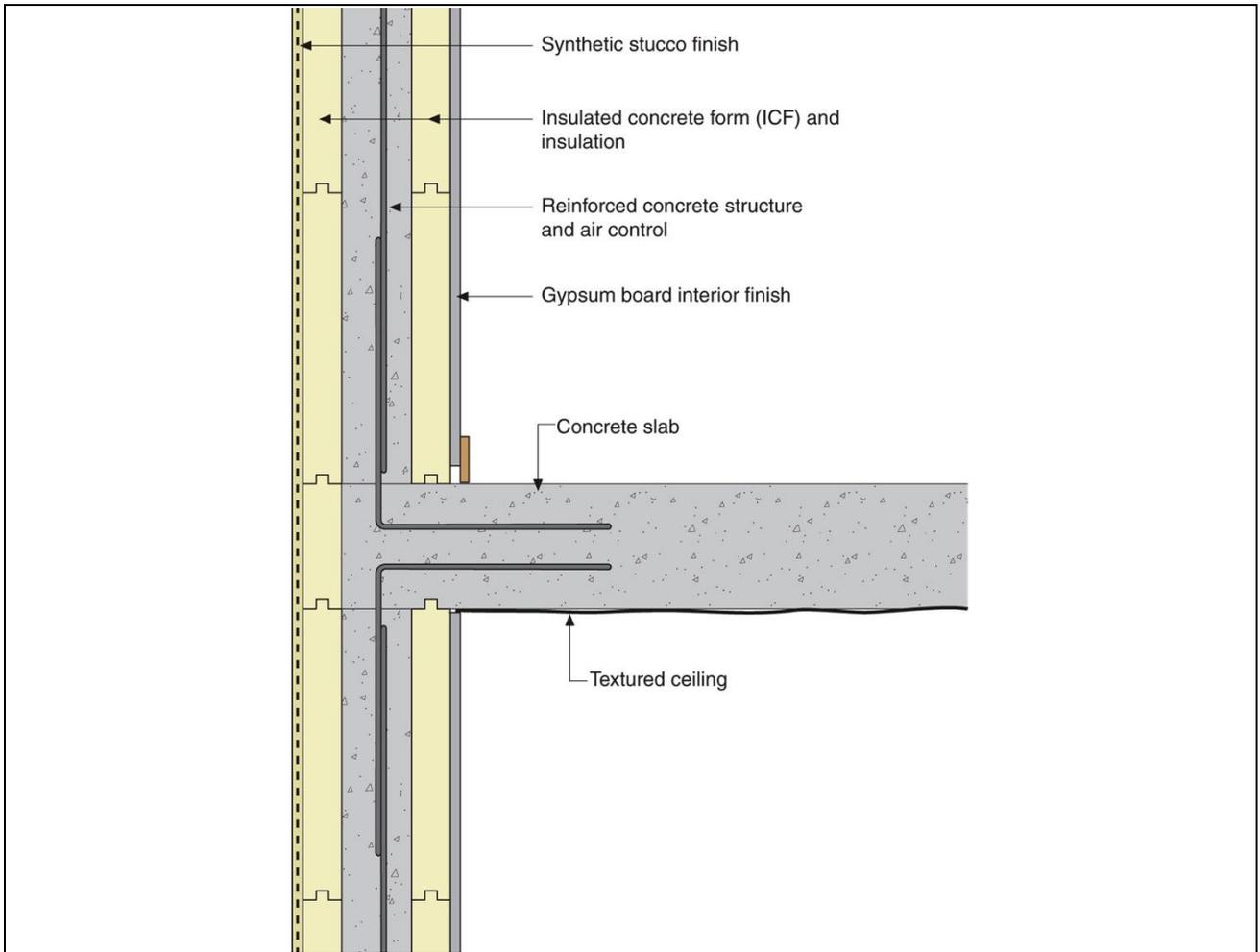
Figure 24: Example floor slab intersection for an ICF with CIP floor.
