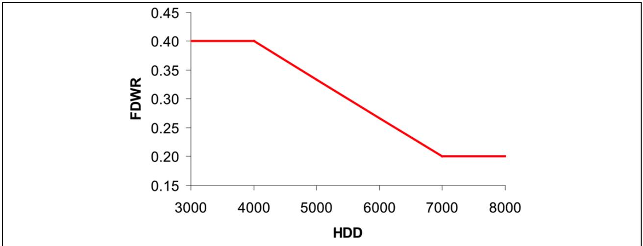
Figure 3: Maximum fenestration-and-door-to-wall ratio (FDWR) varies with the Heating Degree Days (HDD) of the climate under the NECB prescriptive approach.
