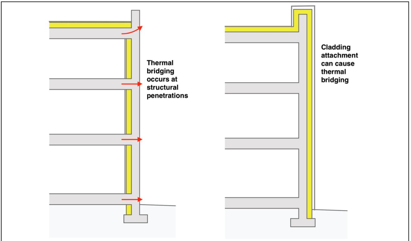
Figure 12: Exterior vs. interior insulated CIP enclosure walls.
