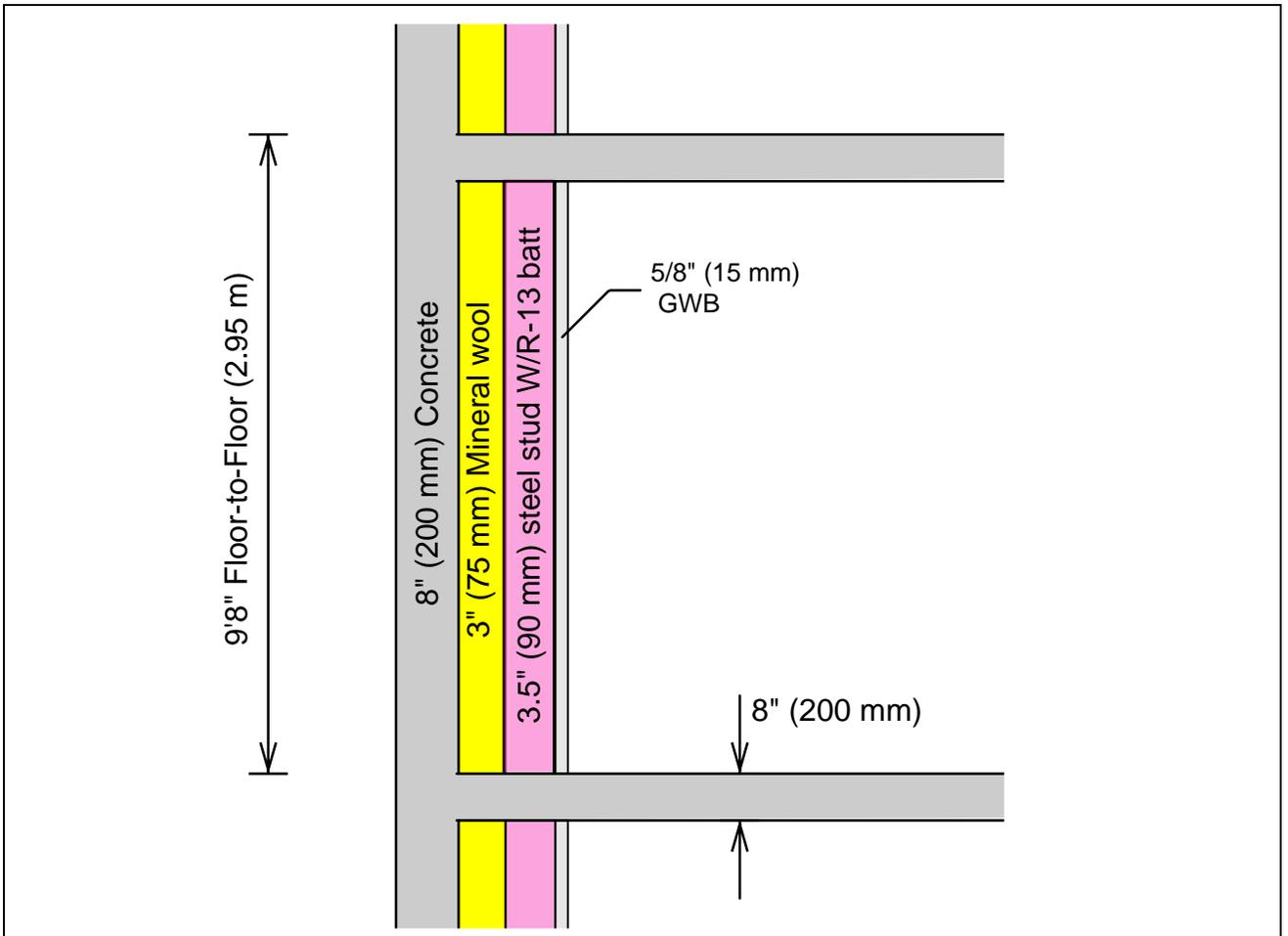
Figure 16: Example interior insulated CIP wall.
