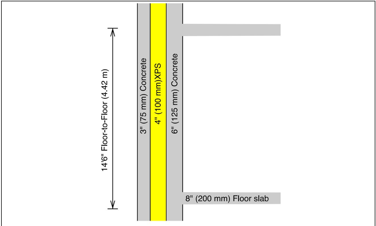
Figure 20: Example double-wythe (sandwich) panel.
