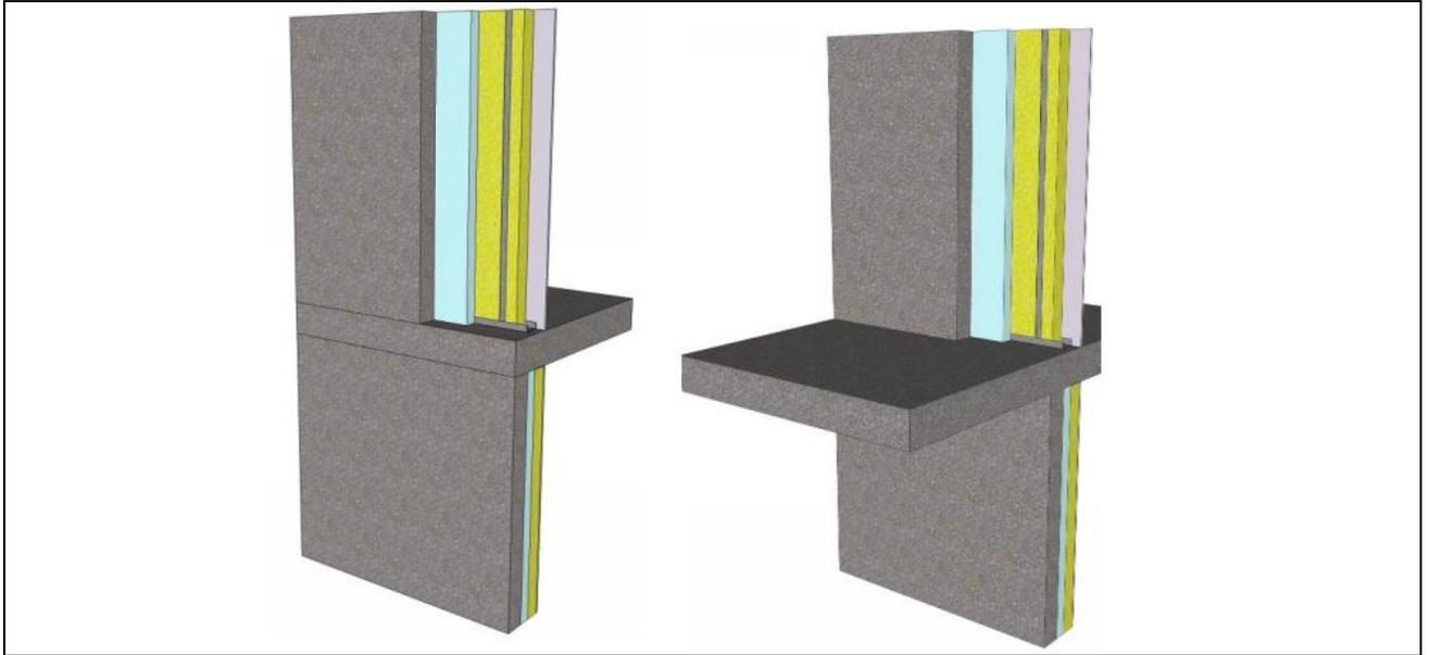
Figure 15: Isometric view of floor slab penetration of interior insulation.
