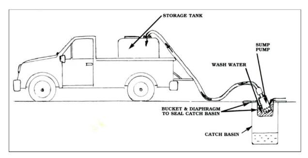
Catch basin sealed with impervious diaphragm sump and pumped into storage tank. (For information on this service contact the BCRMCA.)
