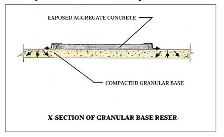
In areas where native soil is impermeable, compacted granular base is required to absorb wash-off water.
