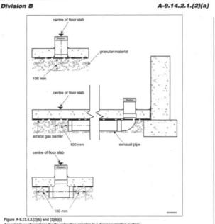
Acceptable configurations for the extraction opening in a depressurization system
